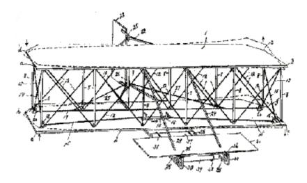
Fig 5: the Wright brothers patented drawing of aeroplane.
